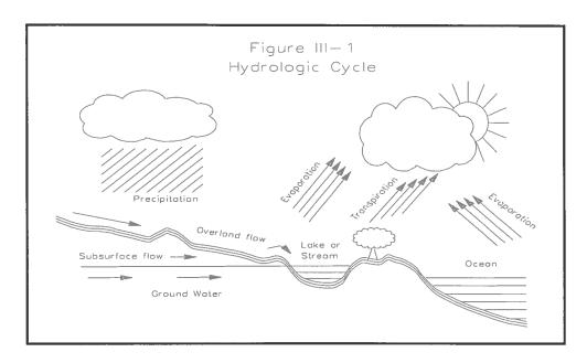
The most important component of the water cycle from the perspective of stormwater management is the overland flow or surface water runoff component. However, as is discussed in subsequent sections of this manual, the techniques which are used to estimate runoff do so by considering the effects of the other forms of water movement.
