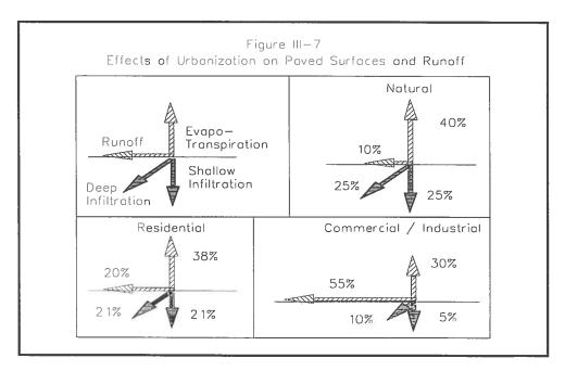
As is indicated in Figure III-7, the increase in impervious area which accompanies most land development activities reduces both infiltration and evapotranspiration rates. This produces more runoff volume than would result otherwise in the natural condition.
