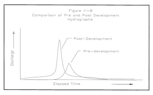
The indicated increases in total runoff volume and peak rate of discharge are the results of decreased infiltration to ground water and decreased interception of rainfall in surface depressions and vegetation. The higher velocities and frequently shorter travel times associated with land development contribute to the higher peak discharge rate and more rapid rise and fall of the runoff hydrograph.
