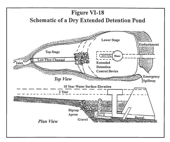
Maintenance of water quality dry ponds is important. Regular mowing, inspection, erosion control, and debris and litter removal are necessary to prevent excessive sediment buildup and vegetative overgrowth. Also, periodic nuisance and pest control could be required. The primary constraints to siting dry ponds are land requirements, topography, and depth to bedrock.
