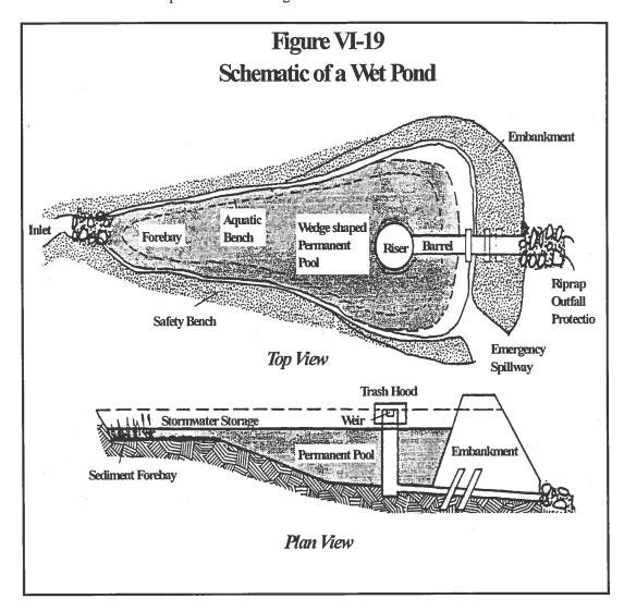
Maintenance requirement for wet ponds include periodic sediment removal (approximately once every 10 to 20 years), mowing, and litter removal. Factors affecting siting include land requirements, soil conditions (soils should not be excessively porous and ground water tables should be relatively high), and topography.
