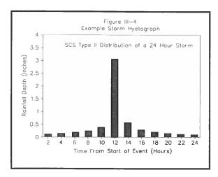
Stormwater and flood control facilities are designed to function properly under specified hypothetical design storm conditions. Design storms are developed from historical rainfall data to represent severe rainfall distribution patterns for given durations (expressed in hours) and frequency (defined in years). Storm duration refers to the length of time over which the precipitation falls. Storm return frequency refers to the average
