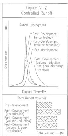
Because it is impractical to entirely avoid increases in total runoff volume, the inevitability of some degree of runoff volume increases must be accepted and the primary emphasis of the stormwater control criteria must be placed on the control of peak discharge rates. In order to minimize the potential for damage, the basic *minimum* stormwater runoff control criteria to be applied is that post-development peak discharges must not exceed pre-development discharge rates.
