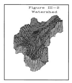
For the purpose of hydrologic modeling and stormwater management planning, watersheds or drainage basins are frequently divided into smaller drainage areas which nest inside and together form the complete watershed. These small, component areas of a watershed are frequently referred to as subbasins.
