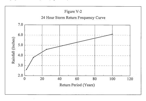
The Beaverdam Branch Watershed Stormwater Management Plan requires that stormwater management/control systems demonstrate the ability to adequately control runoff from storms with the following return frequencies and associated volumes.
