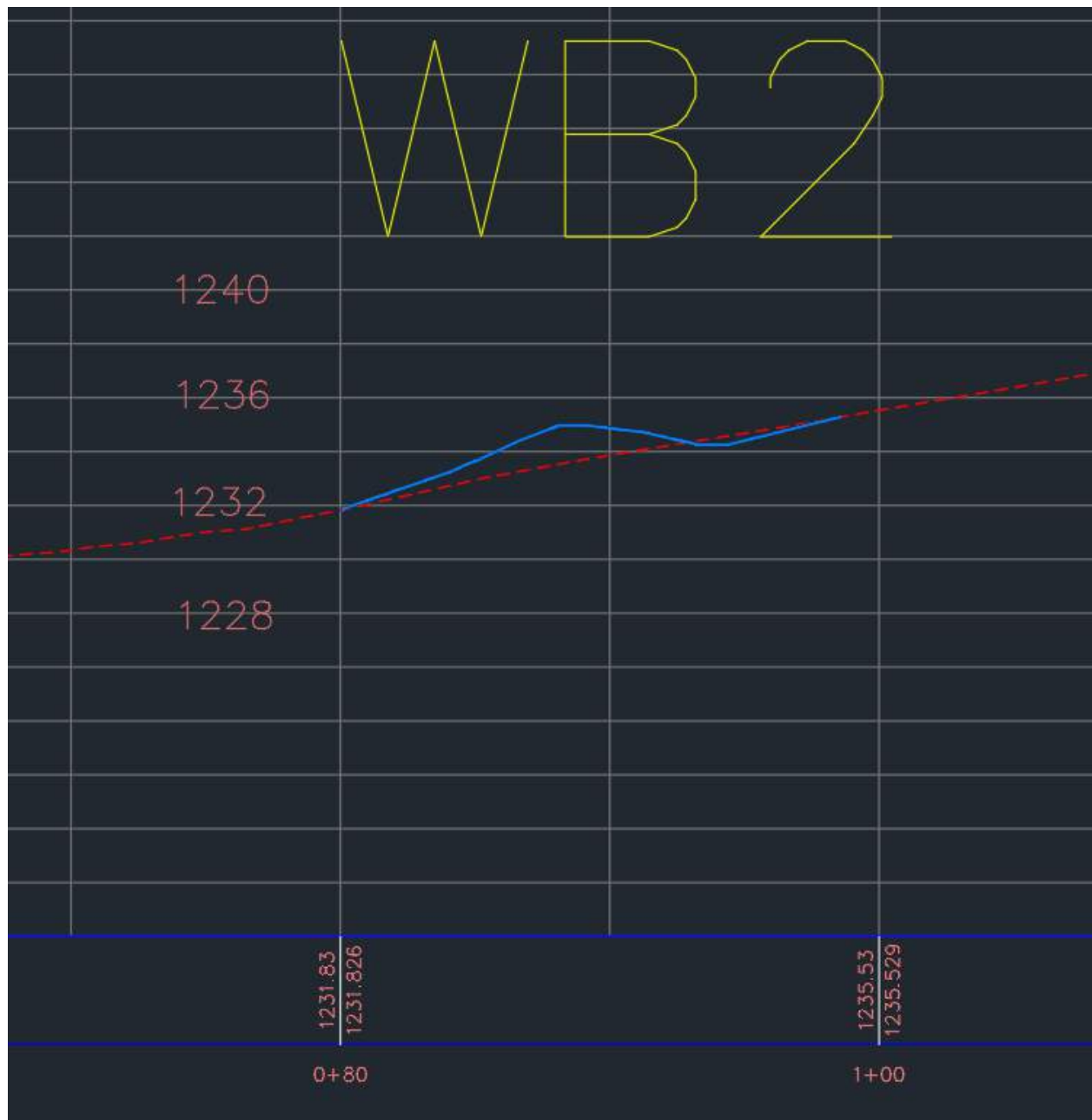
Figure E.7. Location 2 Profile View of Existing and Proposed Ground Elevation
