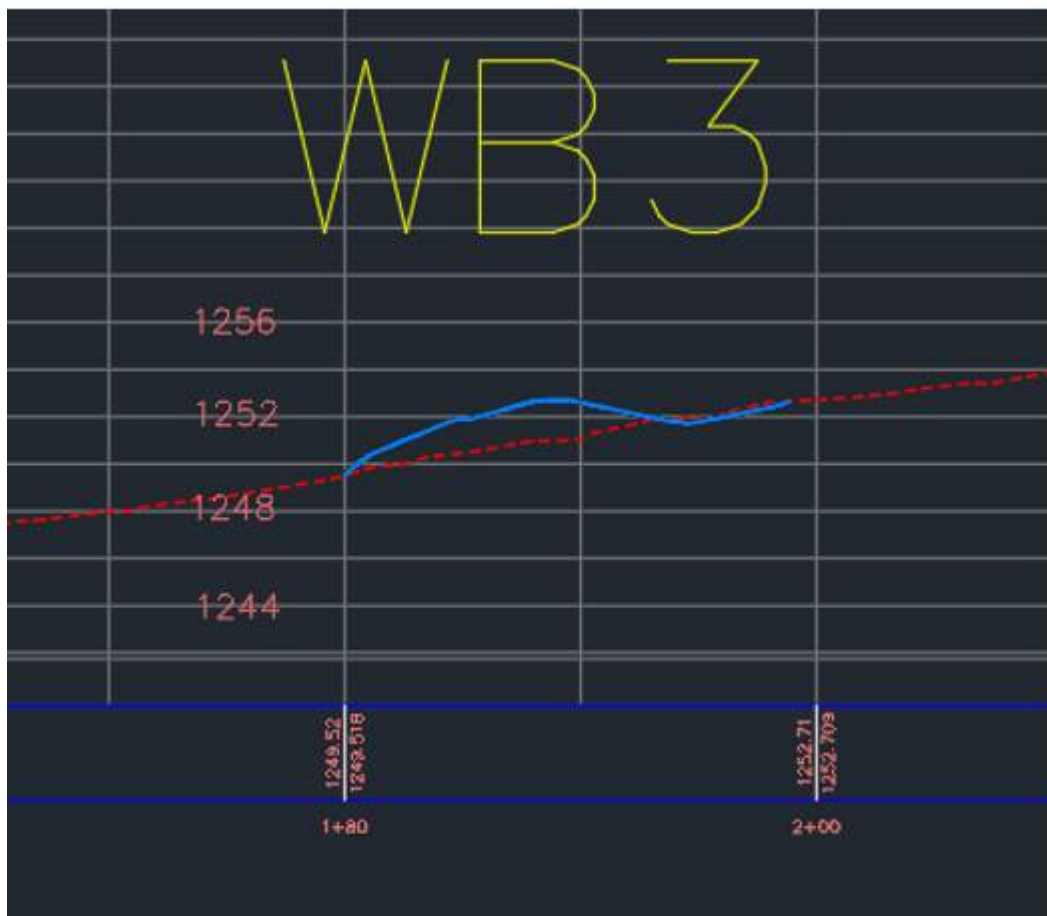
Figure E.10. Location 3 Profile View of Existing and Proposed Ground Elevation
