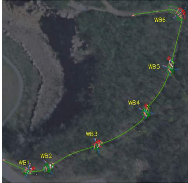
Figure 9.6. Overall Trail Structure Civil 3D Alignment
