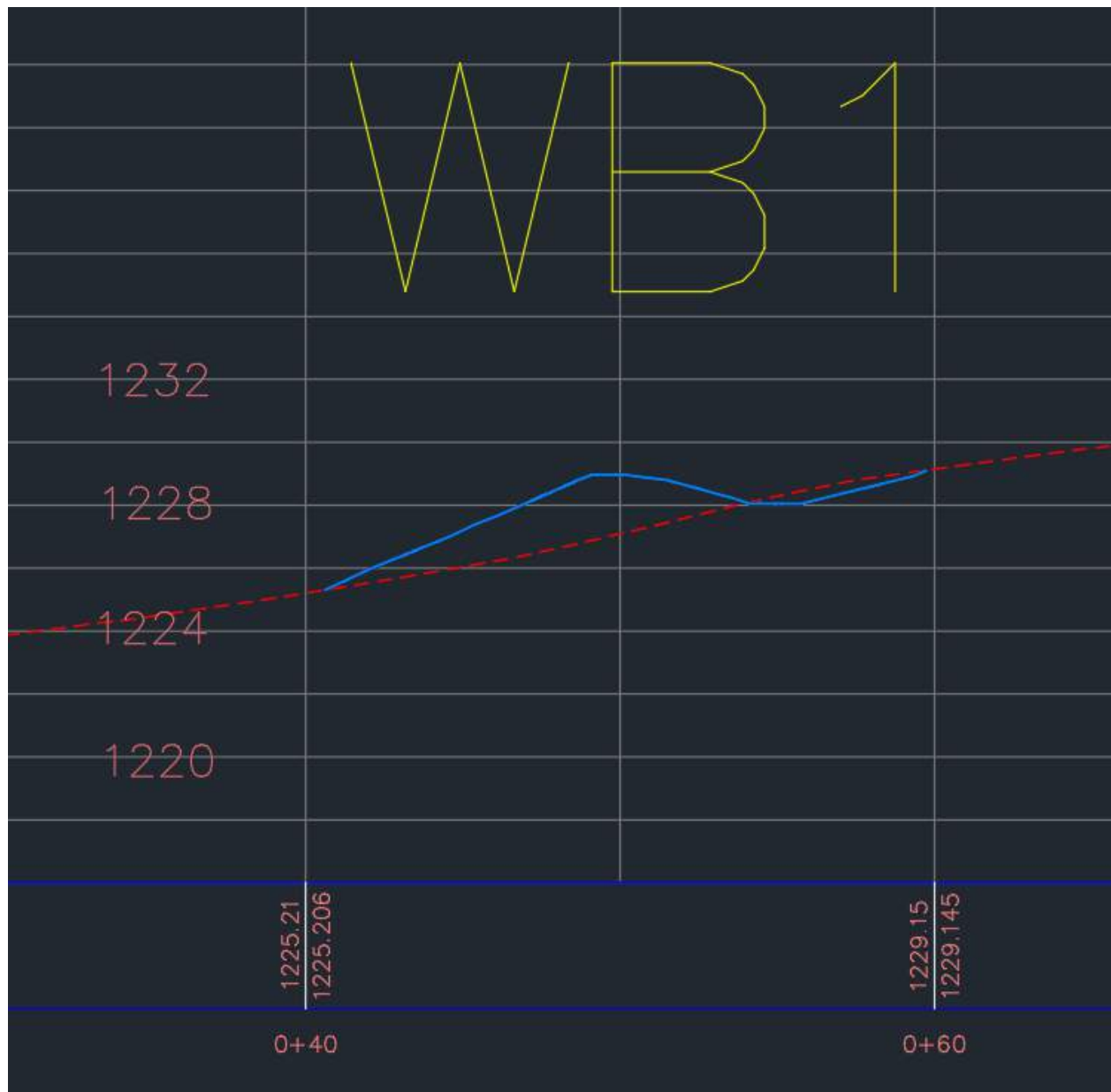
Figure E.4. Location 1 Profile View of Existing and Proposed Ground Elevation
